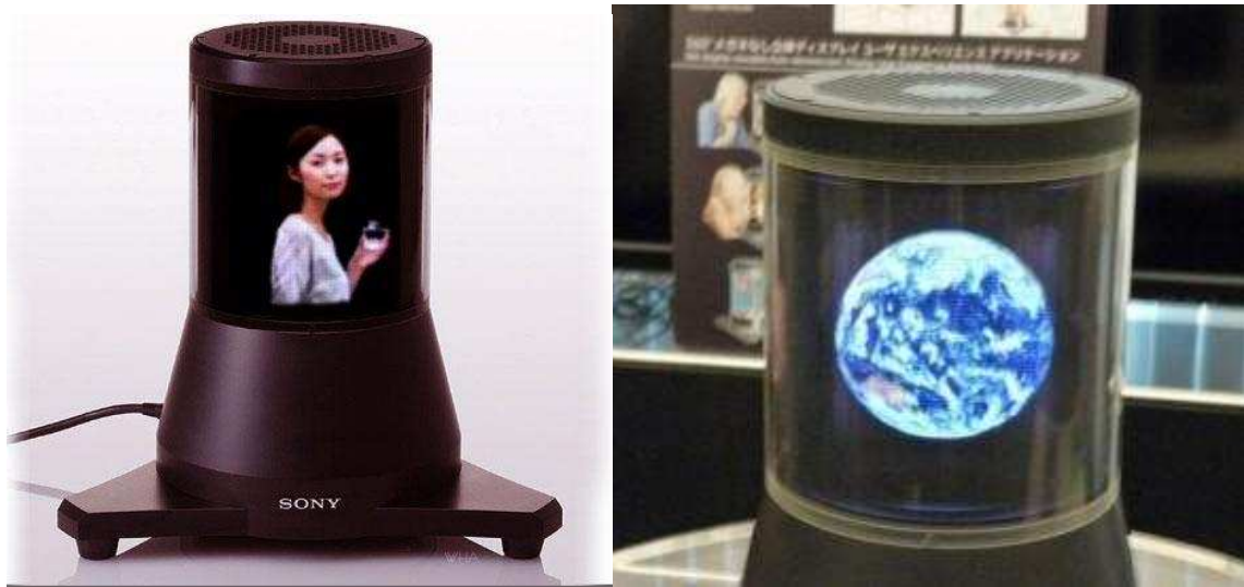
Figure 1.3 The Sony RayModeler prototype: holographic 3D display based on mechanical LED rotation.
