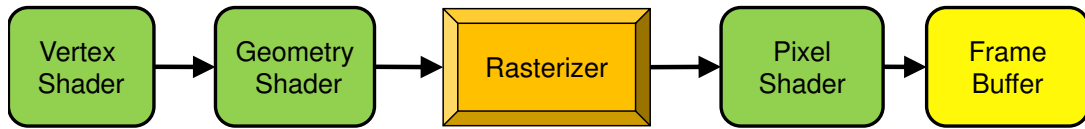
Figure 3.2 The Shader Model 4.0 programming pipeline. All green ovals are programmable units. Note only Rasterizer is a non-programmable unit in SM 4.0
