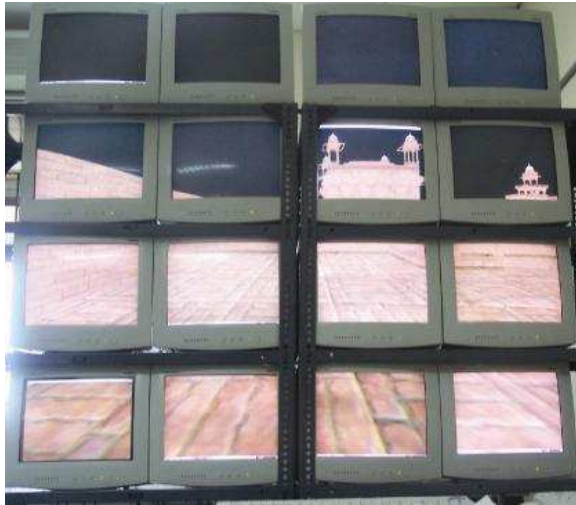
Figure 5.18 A 4 \times 4 display wall showing the Fatehpur Sikri model. The combined resolution is 12 mega pixels.
