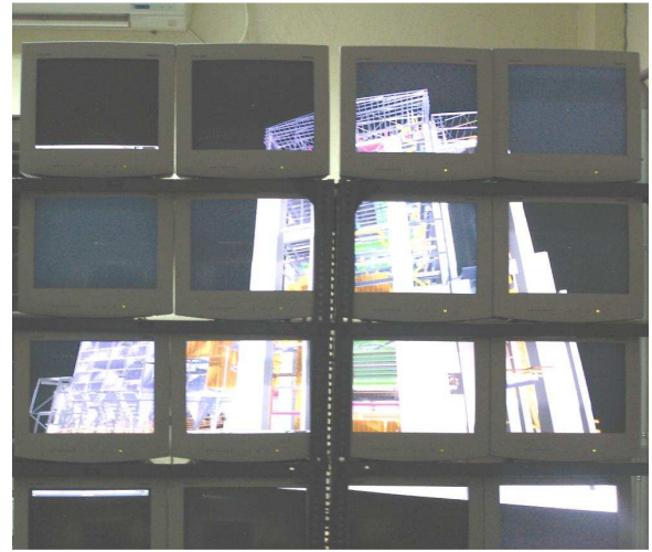
Figure 5.19 A 4 \times 4 display wall showing the Powerplant model. The combined resolution is 12 mega pixels.
