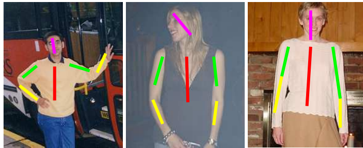
Figure 1.1: Pose estimates by HPE algorithms. The six upper body parts, estimated by the algorithms, are color coded as pink for head, red for torso, green for upper arms and yellow for the lower arms.
