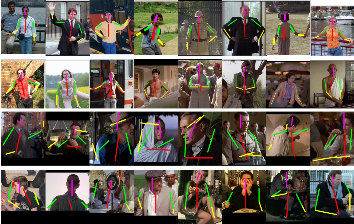
Figure 4.9: Example evaluations. The pose estimates in the first two rows are correctly classified as successes by our pose evaluator. The last two rows are correctly classified as failures. The pose evaluator is learnt using the regime B and with a CPC threshold of 0.3. Poses in rows 1,3 are estimated by Eichner and Ferrari [26], and poses in rows 2,4 are estimated by Yang and Ramanan [103].
