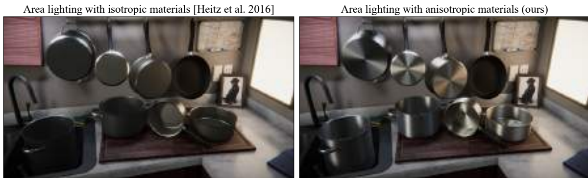
Figure 4.1 Real-time area lighting with Linearly Transformed Cosines (LTCs) in a commercial game engine. Our LTC approximation for anisotropic materials takes 0.7 ms at 1080p resolution on an NVIDIA RTX 2080 GPU.
