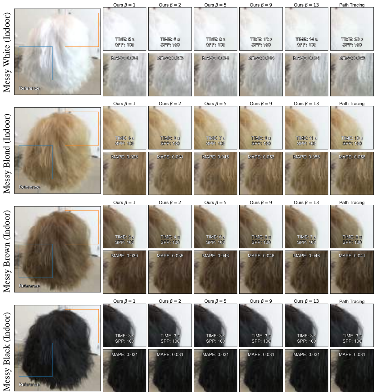
Figure 6.5 Equal spp (100 spp) renders of our method for \beta = 1, 2, 5, 9, 13 compared to path tracing. For white hair, our method with \beta = 1 achieves one-third the error in one-fourth the time. These metrics approach path tracing with increasing \beta . For darker hair, the gain is less pronounced but still significant. Our method behaves equivalently to path tracing on black hair.
