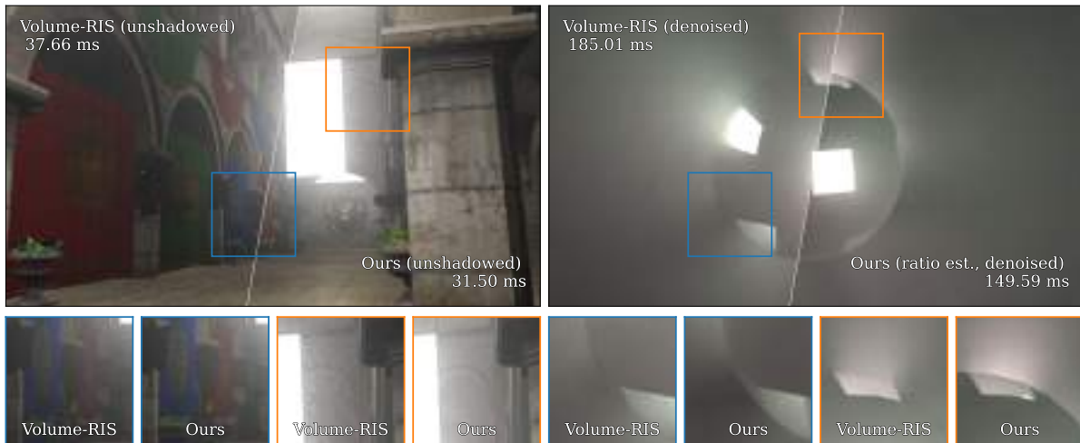
Figure 5.1 We present a semi-analytic method for interactive single-scattering in homogeneous media with polygonal area lights. Our method achieves biased but noise-free renderings and better performance compared to Volume-RIS [47]. This figure shows equal-time renderings of two scenes, Sponza (left) with four area lights and a spherical light shaft (right) with two area lights inside the sphere. Our core unshadowed method (left) is completely noise-free, while Volume-RIS exhibits noise especially near the area light. Our method with the ratio estimator formulation for shadows (right) can handle volumetric shadows due to light shafts, rendering plausible light beams. Note that we denoise the entire image for Volume-RIS and only shadows of our method for the figure on the right.
