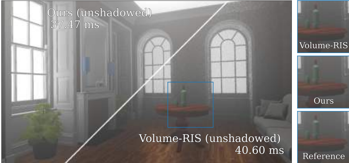
Figure 5.2 Equal-time ( \sim 40 ms) comparison of our semi-analytic unshadowed single scattering with Volume-RIS. Thanks to our use of analytic in-scattered and surface radiance (Eqs. 5.4.3, 5.4.2) and deterministic quadrature for the air-light integral (Eq. 5.15), we obtain noise-free renderings.
