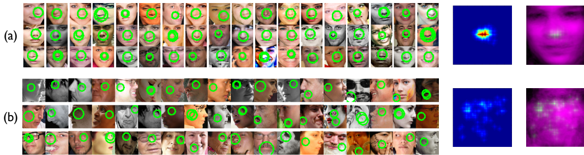
Figure 3.3 Spatial Context of visual words: (a) and (b) shows the location of two visual words in different images. Notice how the visual word in (a) is highly localized with consistent locations while the word in (b) appears at random locations (left). The global distributions of each visual word over the entire database (middle) is used to weight their occurrences in individual exemplars. Its overlay on the mean exemplar face (right), shows strong localization for stable words. Unstable words occurs at diverse locations and are down weighted.
