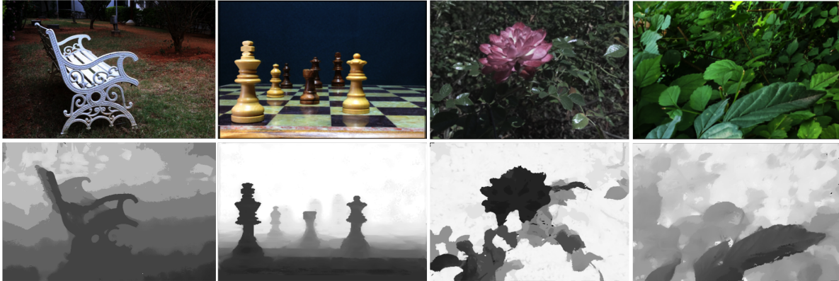
Figure 4.5 Left-to-right: In-focus image F_{\mathcal{I}} and focus map \mathcal{I} for focal stacks captured using Canon EOS 70D, Canon EOS 1100D, Lytro Illum and the Apple iPhone 6.
