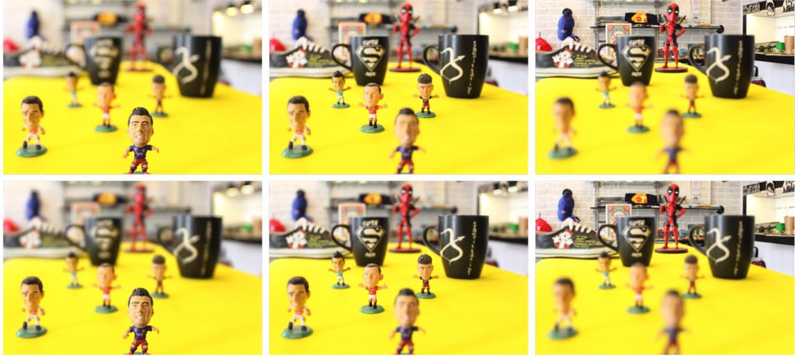
Figure 4.11 Reconstructed Focal Slices 2, 9 and 18 for a focal stack using our representation and refocusing algorithm. The top-row shows the images captured using a DSLR and the bottom row shows our reconstructed images.
