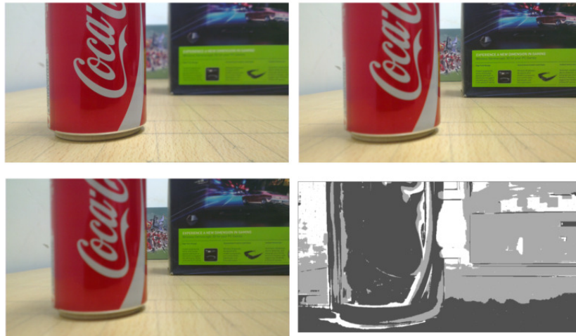
Figure 6.8 The focal stack at a certain C^i consisting of three focal slices, along with the sharpness index map built over the stack.
