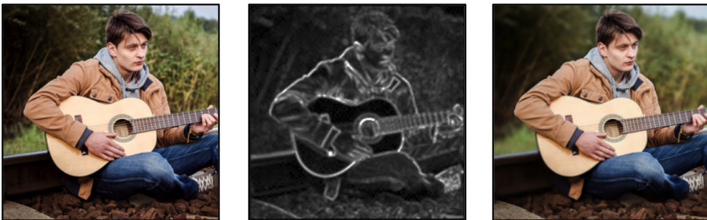
Figure 5.1 Out proposed framework for single-image portraiture. Left: A narrow-aperture portrait image [25] with low defocus in the background. Middle: The composite focus measure [107] computed over the portrait image (contrast enhanced for visualization). Right: A wide-aperture result produced using our method.
