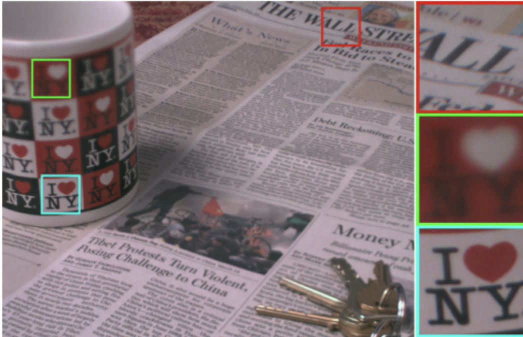
Figure 2.3 Deconvolved extended depth-of-field image from Nagahara et al. [81] where all pixels are reconstructed to be in-focus.
