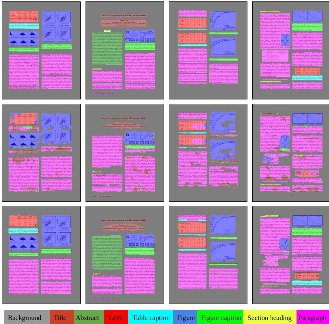
Figure 4.13 Comparison with state-of-the-art techniques in page-level segmentation. Segmentation regions are overlaid with the original images. First row: ground truths, Second row: segmentation results by MFCN, Third row: segmentation results by DeepDocSeg and Fourth row: colors used to represent segmented regions.
