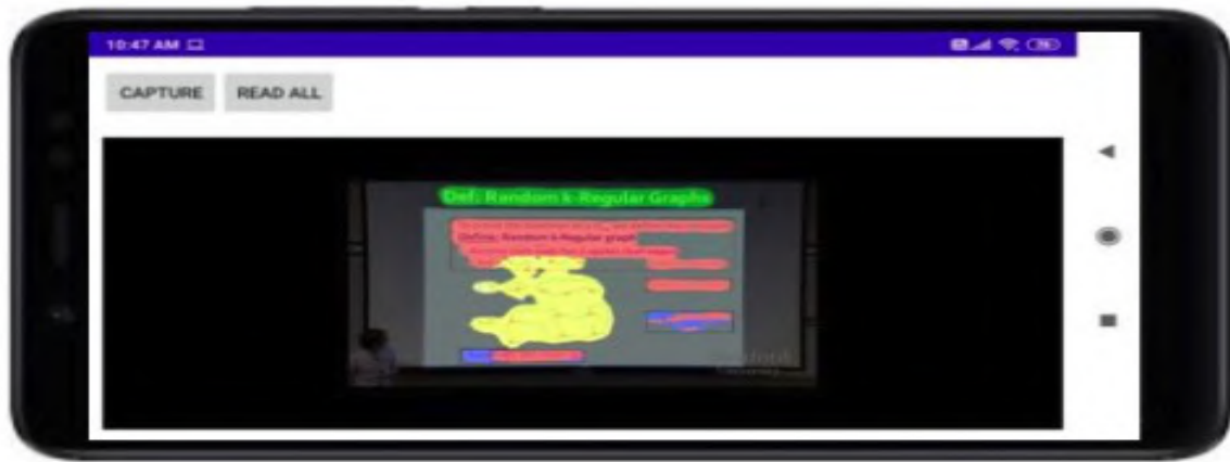
Figure 6.5 The user interface of the developed mobile application. The mobile screen displays the camera-captured slide image. Various colors highlight the slide’s logical regions for better visualization. The READ ALL button plays generated audio sound corresponding to the slide’s content.
