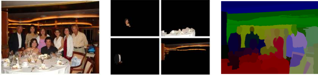
Figure 3.3: Visualizing selective search features: From left-to-right: Original image; four sample mask images from Multi-scale Combinatorial Grouping [20] (binary masks overlaid on the image for visualization) and dimensionality reduced image of selective search features ( g_i ) used for encoding class agnostic semantic information. Notice how regions belonging to an object get grouped together representing approximate semantic information in the scene.
