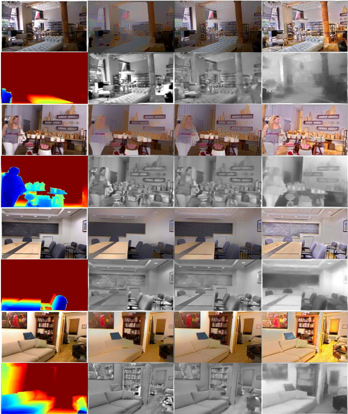
Figure 2.8: Qualitative results on NYUv2 dataset [210]: Our RGBF-IID results on NYU synthetic focal stacks. For each scene top row from left-to-right is original image, RGBF-IID reflectance, RGBD-IID-Jeon [129] reflectance and RGBD-IID-Chen [60] reflectance. Bottom row is depth (blue closer, red farther) and corresponding shading results. Note how our shading results (second column) are able to capture scene highlights and shadows well without significant reflectance gradations (third column) or over-smoothing (fourth column).
