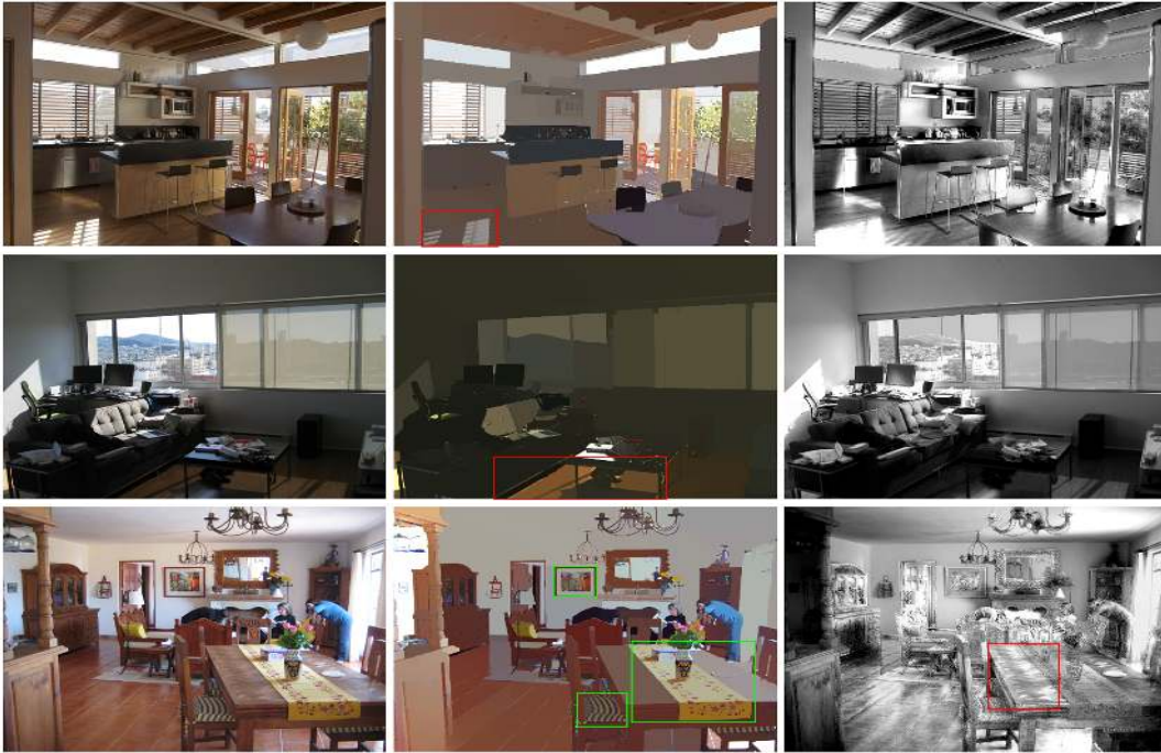
Figure 3.13: Failure cases: Note incorrect decomposition in marked regions with challenging sharp highlights, shadows and fine textures in a colour similar to object. This is an indirect result of our initial shading smoothness and reflectance flatness modelling assumption (L to R : input, reflectance and shading images).
