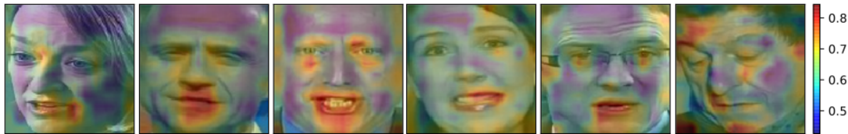
Figure 4.8 Activation maps of the visual encoder shows that the model strongly attends to the lip region while generating speech, despite variations in head pose and lip location.
