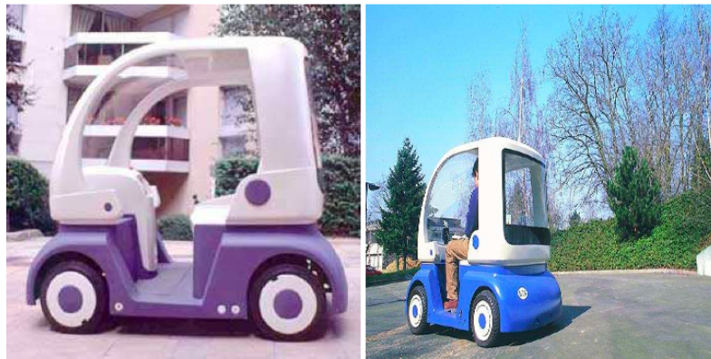
Figure 1.6: Projects like CyCab look at autonomous car following using vision sensors and Multiple View Geometry algorithms. [4]
