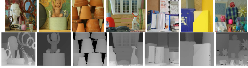
Figure 4.10 Images from the stereo test data set. Top row: original images. Bottom row: output of stereo using pyramid cuts. Image labels, sizes and the number of disparity levels from left to right are: Art ( 1328 \times 1104 , 200), Books ( 1328 \times 1104 , 200), Laundry ( 1328 \times 1104 , 230), Plastic ( 1264 \times 1104 , 280), Bowling ( 1248 \times 1104 , 290), Flowerpots ( 1312 \times 1104 , 251), Moebius ( 1264 \times 1104 , 280).
