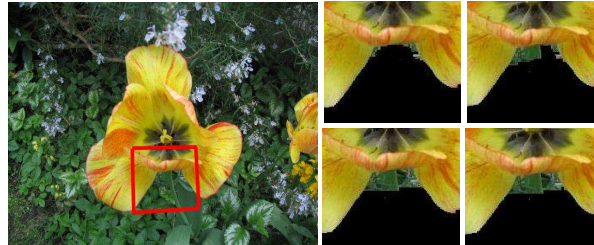
Figure 4.4 Accuracy of segmentation improves as we use pixels from all levels to build the GMMs. Left half shows the image with a window marked on it. Right half shows the segmentation of the marked window when the GMM is built using pixels from: top Left : all images, top right : the largest image, bottom left : the same level only, and bottom right : the smallest image
