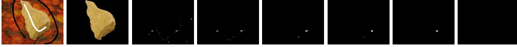
Figure 3.4 First two images are the input sponge image and the segmented output image. The other images shows the errors after 10, 20, 40, 80, 90, 100 iterations of graph cuts for Sponge Image.
