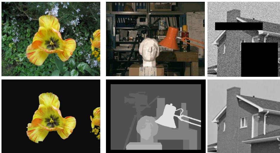
Figure 1.1 Some of the instances of the labeling problems encountered in computer vision. First row: Input images for image segmentation, stereo correspondence and image denoising. Second row: Their corresponding output images.
