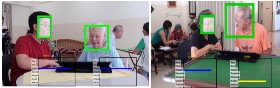
Figure 3.6 Exemplar emotion estimation results. Facial emotions of the PwD and facilitator are correctly identified (left). PwD’s emotion is incorrectly estimated, but facilitator’s emotion is correct (right) (zoom to view).
