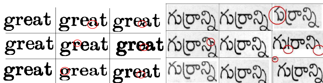
Figure 4.4 Example clusters obtained using LSH over word images. Noisy variants are highlighted in red.
