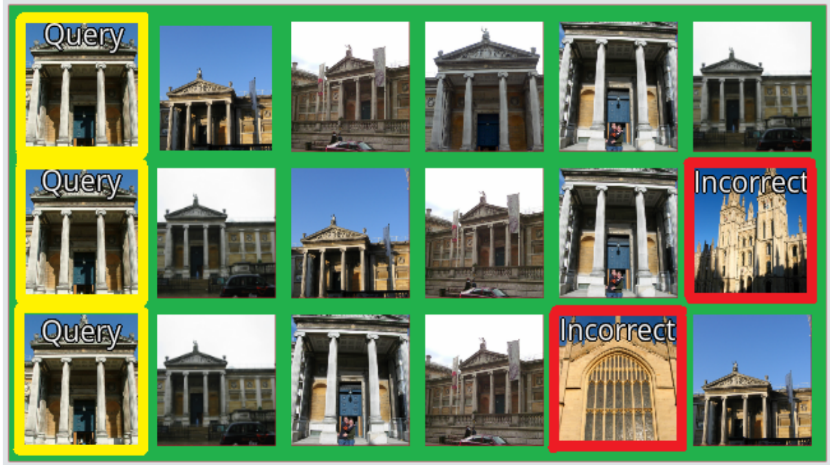
Figure 2.8 Qualitative results on the Oxford Buildings dataset. The yellow boundaries symbolize the query, the green boundaries symbolize correctly retrieved images while the red boundaries represent incorrectly retrieved images for the query landmark.
