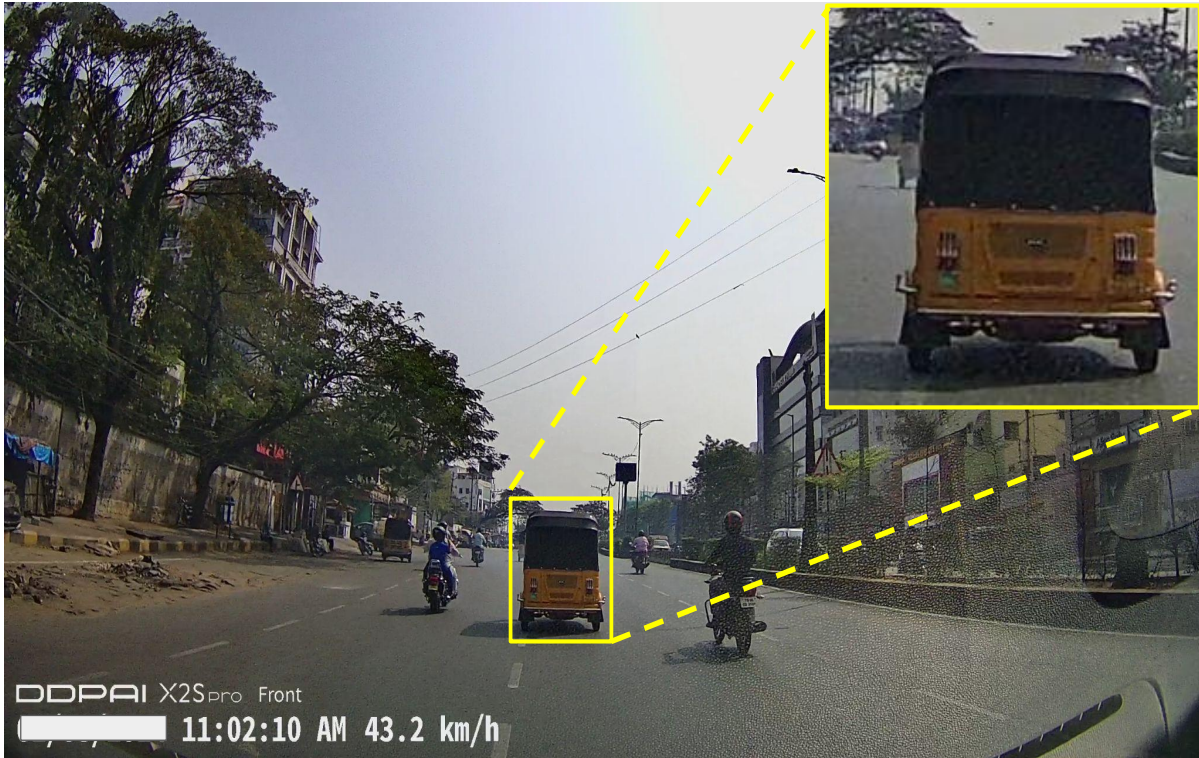
Figure 3.5 HMW scenario from IDD-CRS, with a zoomed-in section highlighting the agent that triggered the alert. The reason for this alert is detailed in Figure 3.2.
