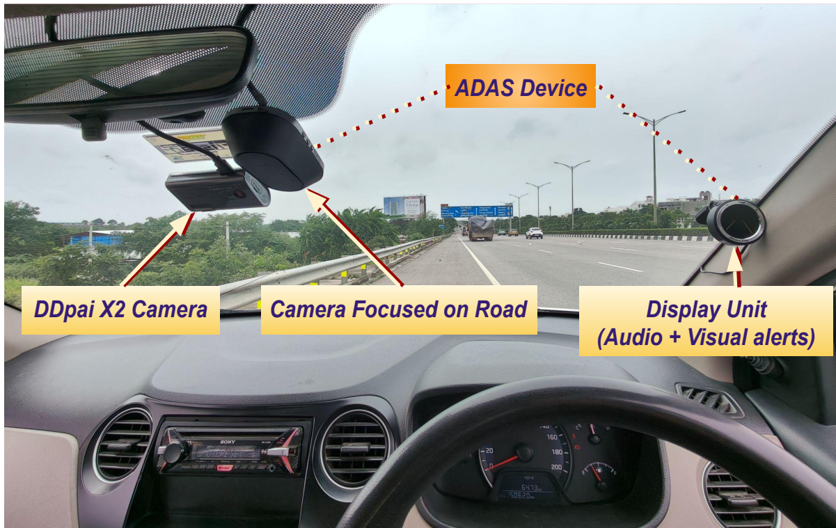
Figure 3.1 Inside view from our car installed with a DDpaiX2 RGB Dash-cam and an Advanced Driver Assistance System (ADAS). The ADAS system comprises (i) a camera installed inside on a windshield and monitoring the road ahead of the vehicle, and (ii) a small display with a buzzer to provide audio and visual alerts to the driver.
