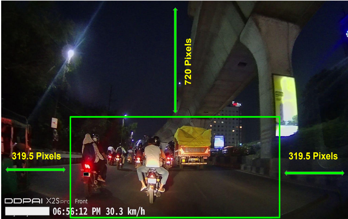
Figure 3.9 Augmented image: The height is reduced to 0.5 times the original height, while the left and right widths are each reduced to 0.12 times the original width.
