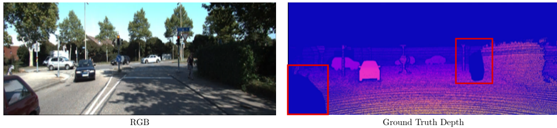
Figure 1.4: Sparsity in depth captured using LIDAR. Post-processing for completion can lead to artefacts as highlighted in red.
