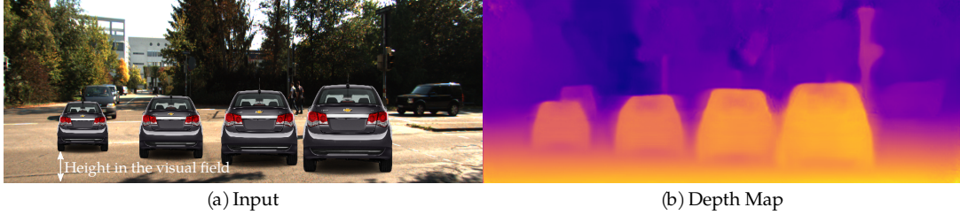
Figure 4.8: (a) is from the KITTI [20] dataset overlaid with car sprites at different heights and sizes. (b) is the depth map estimated using DCNN. Objects higher in the visual field perceptually seem further away.
