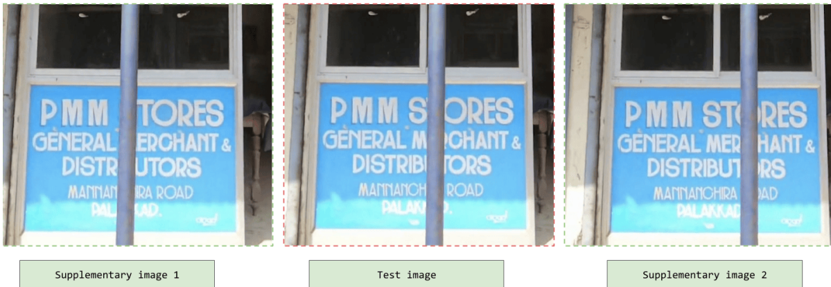
Figure 5.2 Cropped out test image in the middle and the additional images on the left and right help to recognize occluded text.
