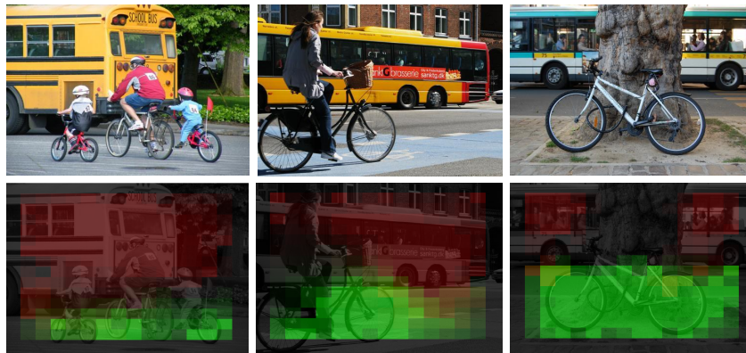
Figure 3.6 Histogram decomposition on Flickr-M2 dataset. LP is solved for two classes bus and bicycle simultaneously. The images and the corresponding weights obtained for their cells using the LP solution are shown. The cells shown in red are weights of bus , while those in green are of bicycle . Higher intensity of the colour represents a value closer to 1. ( Best viewed in colour. )
