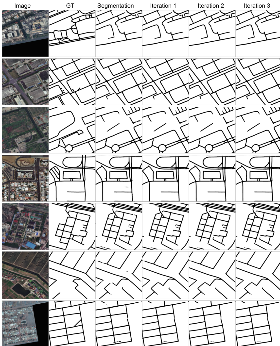
Figure 4.15: Qualitative results of Connectivity refinement over segmentation and orientation learning with LinkNet34 [10] as joint learning module.
