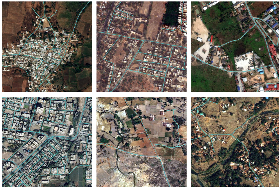
Figure 2.5: Sample images from DeepGlobe [18] Road Dataset with road center lines. Center lines are obtained using skeletonization of ground truth segmentation mask followed by vectorization.
