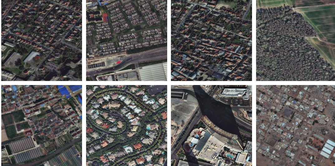
Figure 1.1: Few examples of challenges in the satellite imagery, (a) Occlusion by shadows of trees and buildings, and (b) Visual ambiguity in identifying the roads.
