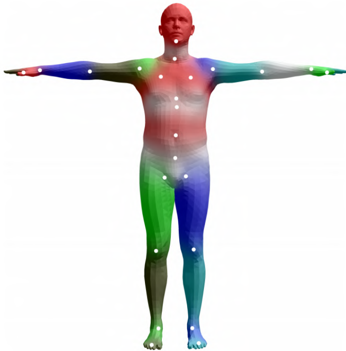
Figure 2.1 SMPL Representation: This figure demonstrates SMPL base human pose representation. This is essentially represented by body pose (3D joint rotation of 23 joints) and body shape (beta parameters). (Image taken from Loper Matthew, SMPL: A Skinned Multi-Person Linear Model, SIGGRAPH Asia [30])
