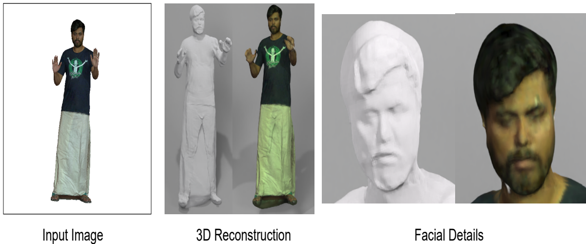
Figure 1.5 Problem Statement: Given a monocular RGB image as input, the final goal is to reconstruct robust photo-realistic 3D humans.
