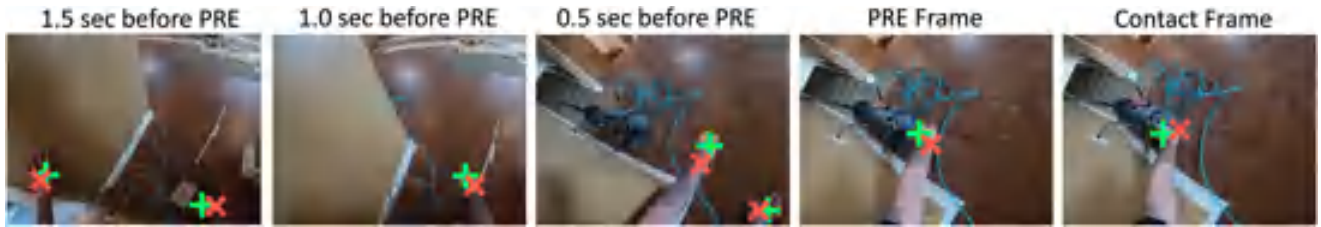
Fig. 28. Qualitative examples of future hands movements prediction using the proposed baseline. The ground truth hands positions are plotted as green crosses, while the predicted hands positions are plotted as red crosses.
