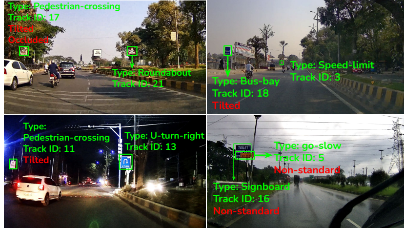
Fig. 2: Frame-level traffic sign annotations in the MTSVD [4]. The dataset contains bounding-box track annotations with multiple attributes like tilted , occluded , etc., and is captured in diverse weather and lighting conditions.
