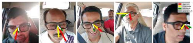
Fig. 9: Qualitative results of DashGazeNet gaze angle prediction on randomly selected samples. Arrow colors represent the following: red: Gaze360 [3], yellow: ETHX-Gaze [20], green: DashGazeNet, and white: ground truth.
