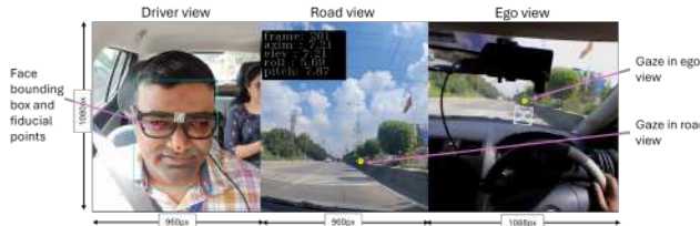
Fig. 2: Overview of the DashGaze dataset. Each frame consists of driver view, road view and ego view. We also provide face bounding box and fiducial points, head IMU data, driver gaze coordinates with respect to the road view, blink and fixation data.
