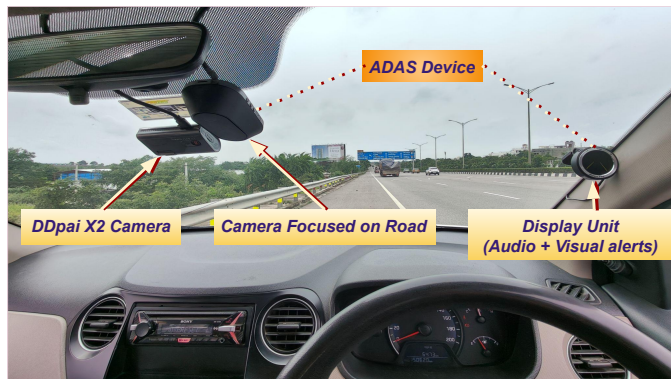
Fig. 1: Inside view from our car installed with a DDpaiX2 RGB Dash-cam and an Advanced Driver Assistance System (ADAS). The ADAS system comprises (i) a camera installed inside on a windshield and monitoring the road ahead of the vehicle, and (ii) a small display with a buzzer to provide audio and visual alerts to the driver.
