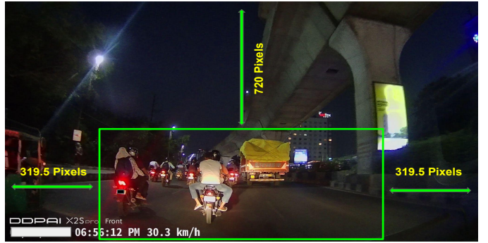
Fig. 6: Augmented image: The height is reduced to 0.5 times the original height, while the left and right widths are each reduced to 0.12 times the original width.
