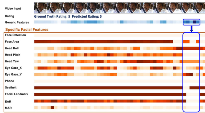
(a) Case I: Driver with attention rating-5. In above figure, we observe that attention probability corresponding to generic features is high for 10% of the total video length. This means driver is attentive in majority of the video and hence the rating-5. Specific facial feature block corresponding to this inattentive region of video show high attention probability for 'Head Roll' and 'Eye Gaze'. This concludes that driver is not looking straight on road for this section of the video and hence the reason for his inattentiveness.
