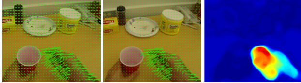
Figure 2: If the camera was static, salient regions in the image for an action recognition task can be computed as parts with moving objects. In egocentric setting, where the camera is also moving, we first cancel the component of flow due to camera motion. We note that the motion of the egocentric camera is 3D rotation for the considered actions. Such motion can easily be compensated by cancelling a 2D homography. Left and center images shows the original and compensated flow. We use the dominant motion direction from the compensated flow and use the component of flow in the direction of dominant motion direction to generate a saliency map (right image). See the text for the details.
